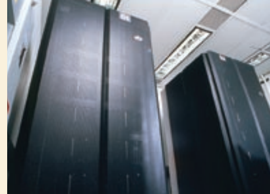
Deep Blue (1997) was based on IBM's RS/6000 SP2 supercomputer, consisting of 30 processors in two towers (shown). The 480 identical custom chess chips (integrated circuits) were key to the system's performance as a chess playing machine. It calculated 200 million positions per second, at times up to thirty moves ahead. Courtesy of IBM Archives, CHM# L062302016
