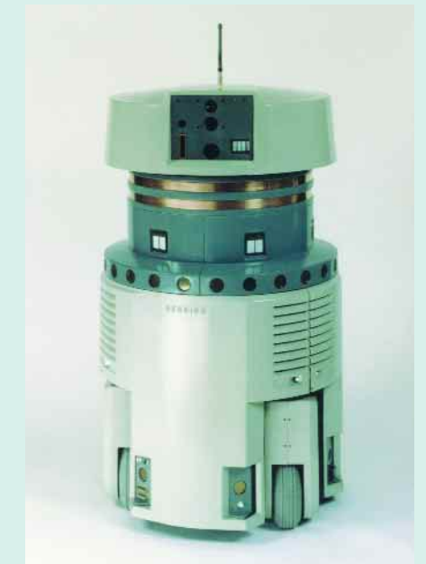
The Denning Mobile Robot, used to guard hallways in areas such as prisons and warehouses, was equipped with sonar and microwave beacons to guide it along
