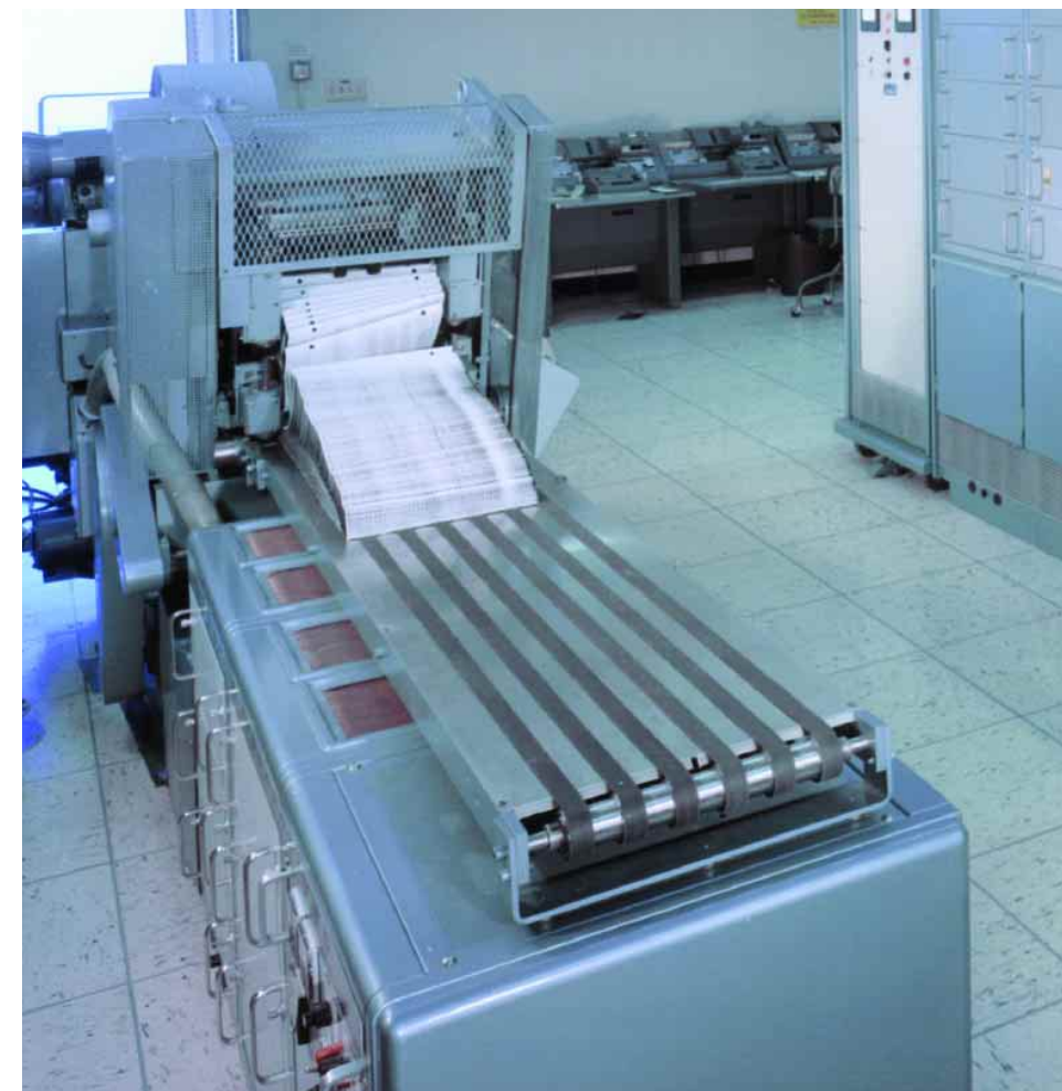
(above) Operator Mona Millings stands at the table where the separated output was delivered from the printer, and at the other end, the large rolls of paper used by the machine. Paper from the rolls could be spliced head to tail so there was no ordinary need for rethreading through the press. A roll lasted about 45 minutes and a special dolly was needed to move the rolls, since at over 200 pounds, they were far too heavy to be moved by hand.
