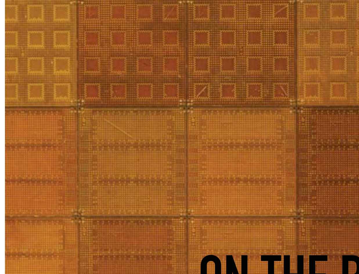
Cray-3 CPU section, Cray Computer Corporation, 1995 Unlike Cray's previous designs, the Cray-3 used unproven technology—gallium arsenide and sophisticated assembly robots to build it
