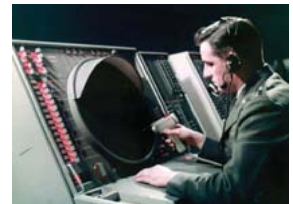
Capt. Charbonneau sits in front of SAGE's situation display console at the Lincoln Labs' Experimental Direction Center, where SAGE testing took place
