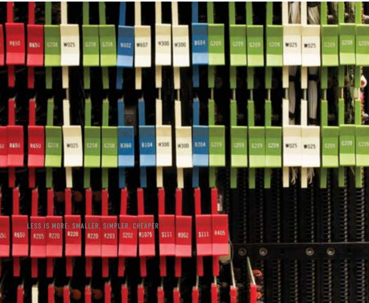
Close-up of DEC PDP-8 flip-chip modules
